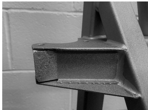
Figure 8 – LWE suspension mounting gusset for increased rigidity.
