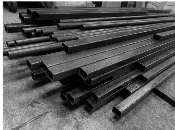
Figure 2 - Selection of tubing used in frame manufacture.
