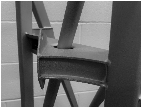
Figure 7 – LWE engine mounting gusset, prevents buckling.
